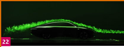
22 The Lightyear o, a Dutch-designed solar car, undergoes wind testing at the Delft University of Technology. In order to use its energy efficiently, this electric vehicle must be as light and aerodynamic as possible to travel forward with least resistance. (p. 45)
